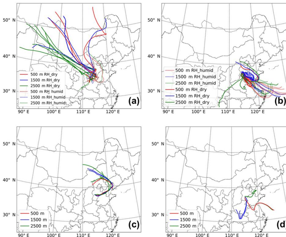
**Figure 9.** 72 h HYSPLIT back trajectories for the cases when the PBL was (a) clean, (b) polluted in the lower PBL, (c) polluted in the upper PBL in the flight on 2 June, and (d) polluted in multiple layers of the PBL in the flight on 6 June. Trajectories at different levels under dry (solid lines) and humid (dashed lines) conditions are shown: 500 m (red), 1500 m (blue), and 2500 m (green) above mean sea level.
