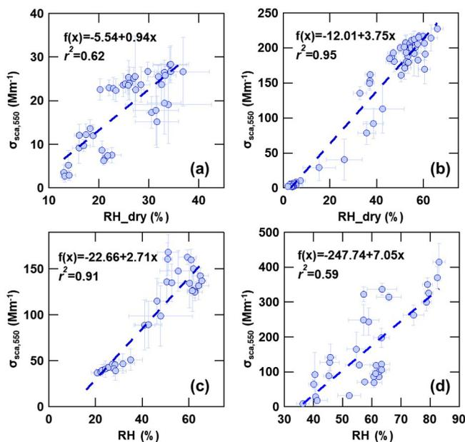
**Figure 8.**  $\sigma_{\text{sca}}$  at 500 nm as a function of relative humidity (RH, in %) for those cases when the PBL was (a) clean and dry, (b) polluted in the lower PBL and dry, (c) polluted in the upper PBL in the flight on 2 June, and (d) polluted in multiple layers of the PBL in the flight on 6 June. The linear regression best-fit lines through the data are shown (dashed lines). The regression relationships and coefficients of determination are given in each panel.
