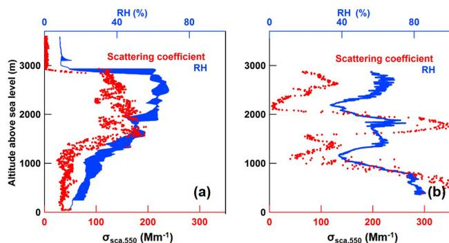
**Figure 7.** Vertical distributions of  $\sigma_{\text{sca}}$  at 550 nm (red) and relative humidity (RH, blue) for the enrichment of aerosols in the upper layer of the PBL on 2 June in LC (a) and in multiple layers of the PBL on 6 June in JL (b).
