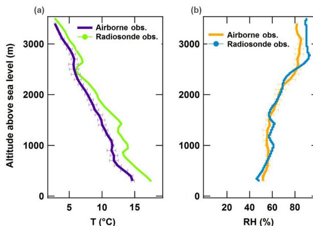
**Figure 2.** Vertical profiles of temperature ( $T$ , a) and relative humidity (RH, b) from radiosonde and airborne measurements made on 8 May 2016 over the Xingtai supersite. Horizontal bars represented standard deviations.
