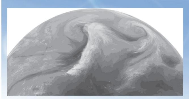
This is a "false color" image. Water vapor absorbs and emits energy. You can tune an instrument to only "see" the wavelengths where water vapor absorbs and emits energy
