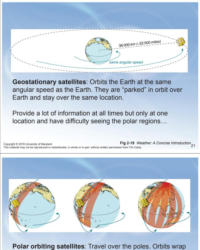
**Polar orbiting satellites**: Travel over the poles. Orbits wrap around the Earth. Need to travel quickly to provide cover the globe. Can be very high resolution because they orbit closer to the surface than geostationary satellites
