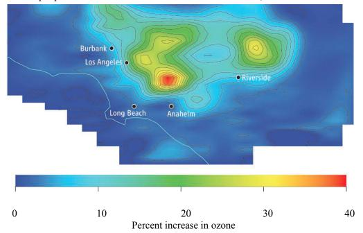
**More pollution?** The difference between photochemical simulations for 27 to 29 August 1987 in California obtained with and without including the OH source from the reaction of electronically excited  $NO_2$  with  $H_2O$  described by Li et al. (2008). The figure shows the percentage increases in  $O_3$  due to this new chemical process.
