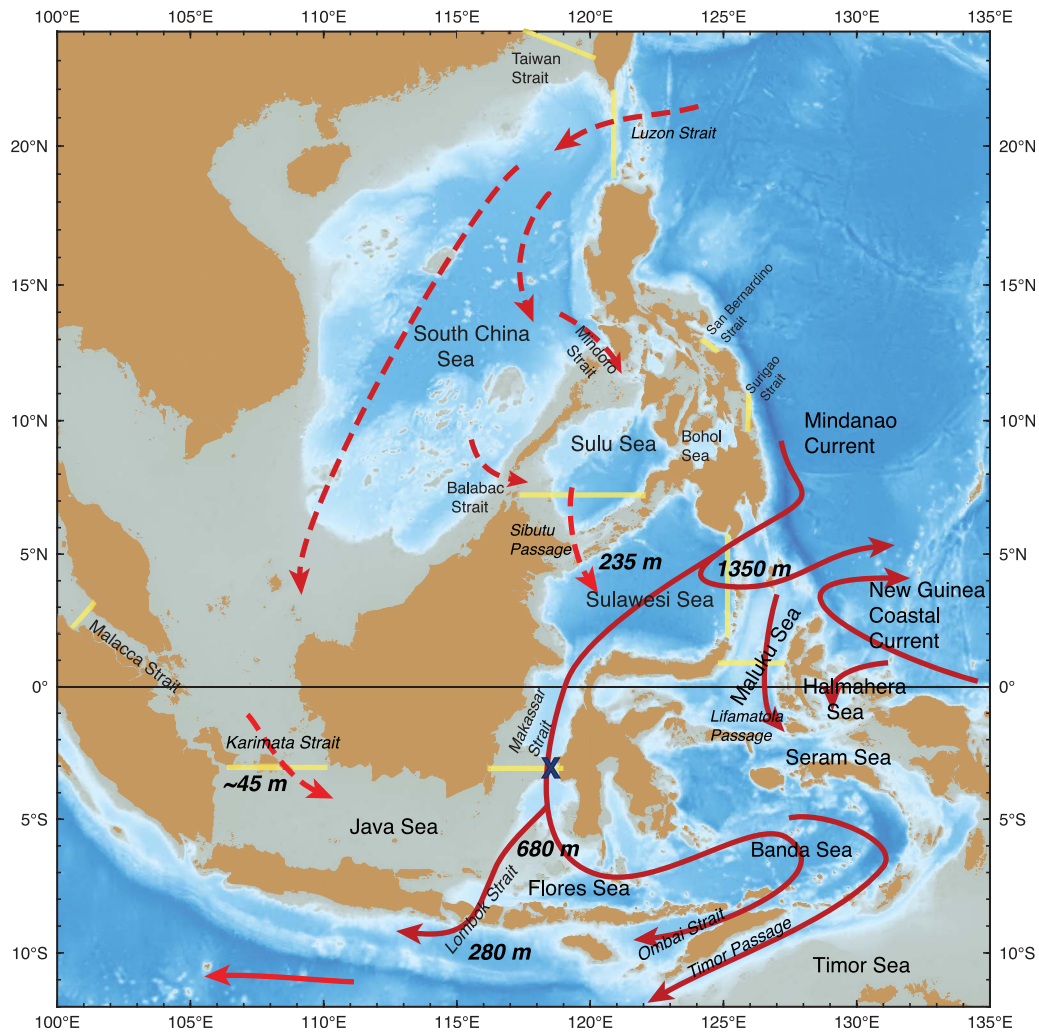
Figure 1. Schematic of the South China Sea throughflow (dashed red arrows) and the Indonesian throughflow (solid red arrows) circulations. Topographic sill depths are given in black italics. The X indicates Makassar Strait mooring site.
